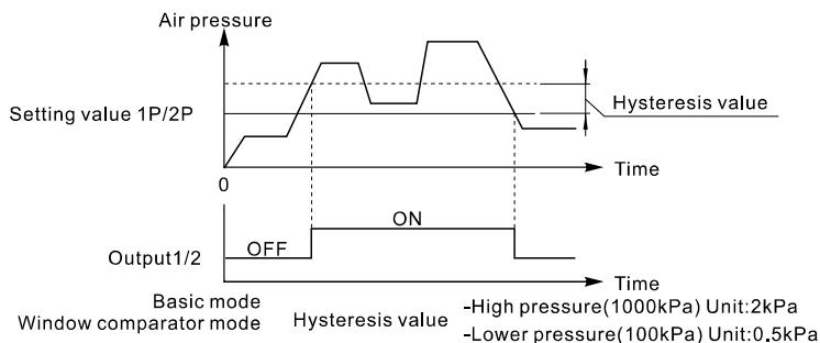
2. Hysteresis mode: Set the pressure value 1H/2H/1L/2L. When the applied pressure value is greater than 1H/2H, the display will ON. When the applied pressure is less than 1L/2L, the display will OFF.
