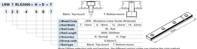
[Note1]When selecting rails and bearings, the different pairing codes can change the uints preload.
